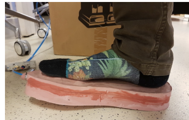
Fig. 8. The sole in flexion state inflated with 2 bar at full weight
