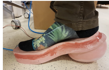
Fig. 7. The sole in extension state inflated with 2 bar at full weight
