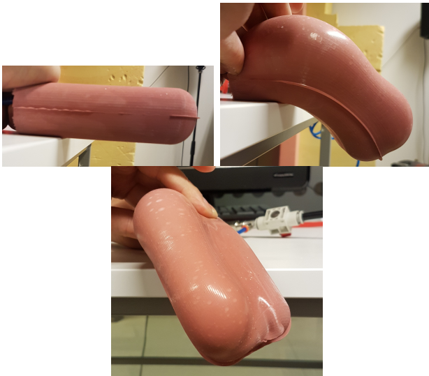
Fig. 7. Pictures of Iteration 4. Top left shows 0 bar pressure, top right shows approx 1 bar pressure, and bottom picture shows what rotation that was achieved from 1 bar pressure.
